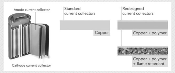
cientists at Stanford and SLAC redesigned current conductors, thin metal foils that distribute current to and from electrodes, to make lithium-ion batteries lighter, safer and more efficient. They replaced the all-copper conductor, middle, with a layer of lightweight polymer coated in ultrathin copper (top right), and embedded fire retardant in the polymer layer to quench flames (bottom right).
