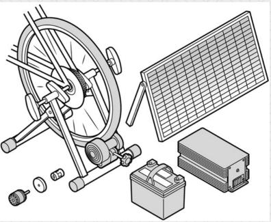
the motor—originally intended to motorize a skateboard and now acting as a generator—to a three-phase bridge rectifier. The output of the rectifier in turn is connected to my battery through a Drok meter. This meter allows me to monitor the voltage, current, wattage, and total energy produced.
